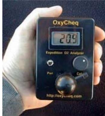
The **OxyCheq Expedition Oxygen Analyzer** uses a removable cap with a built-in flow restrictor. Although not necessary, you can also attach a 2-3 lpm flow restrictor to the sensor cap/flow restrictor if desired.
