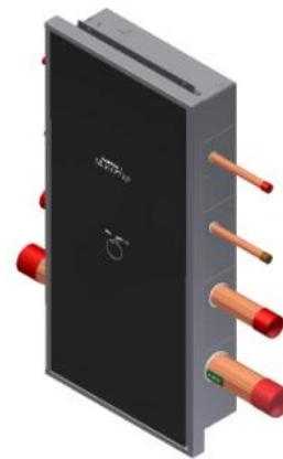
Shown above EZ42ASB2NSB3OSB4VSS 4 valve box with gauges ½” Medical Air, ½” N 2 O, ¼” Oxygen, all with E Z Backfeed on the right side of valve and 1” Medical Vacuum
